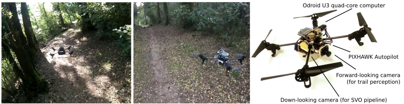
Fig. 8: Images from preliminary field testing. Left: the Parrot ARDrone controlled by a laptop. Center, right: the standalone quadrotor with SVO and onboard processing [34].
