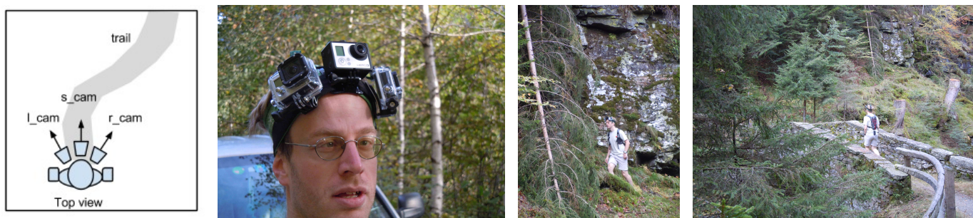
Fig. 4: Left : stylized top view of the acquisition setup; Right : our hiker during an acquisition, equipped with the three head-mounted cameras.
